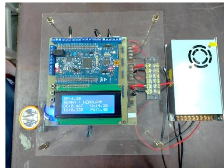
Figure 9. System implementation for charging headlamp
