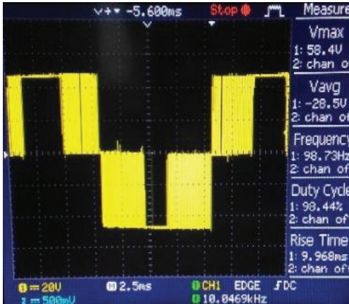
FIGURE 6. The wave of inverter output.
