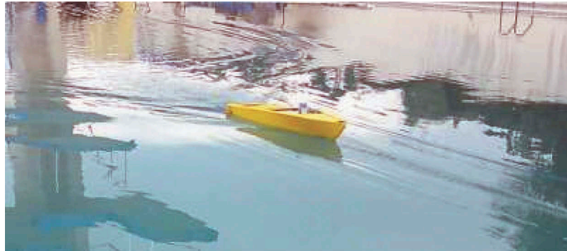
Figure 4. Experimental condition on the 25-m water basin, ship models were towed by electric motors.
