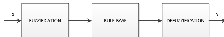
Figure 5. The basic structure of the fuzzy logic controller system
